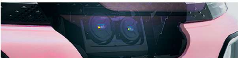
DC Fast Charging Port / AC Slow Charging Port
